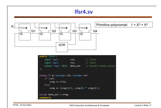
Here is the implementation of a 4-bit LFSR of the primitive polynomial
