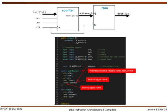
A simple sinewave generator can be designed with combining **counter.sv** and **rom.sv**. The counter produces the address of the ROM, and the output is the sine (or cosine) values. The frequency of the output sinewave is determined by **incr[7:0]**. If incr = 1, then the sinewave period is 256 x clock period. In general, the output sinewave frequency is:
