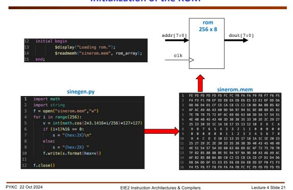
ROM needs to "programmed" or configured with original contents. In SystemVerilog, the **\$readmemh(.)** function allows the ROM to be loaded with the contents stored in a file with numbers stored as hexadecimal code as
